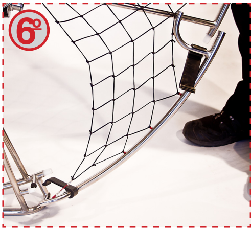
The bar is now fully detached, joined by the net to the top frame part.
